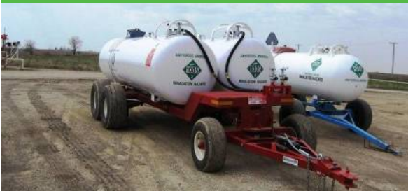
Twin 1,500 Gallon Ammonia Nurse Tanks
